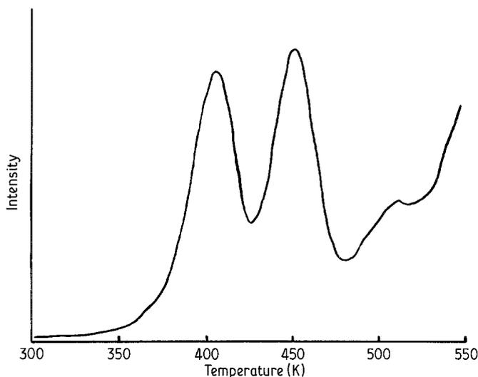
Figure 1 Thermoluminescence spectrum for tricalcium aluminate.
